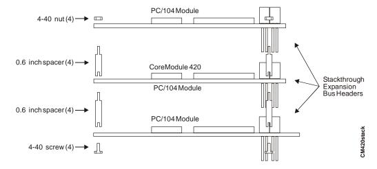
Figure 2-1. Stacking PC/104 Modules with the CoreModule 420
